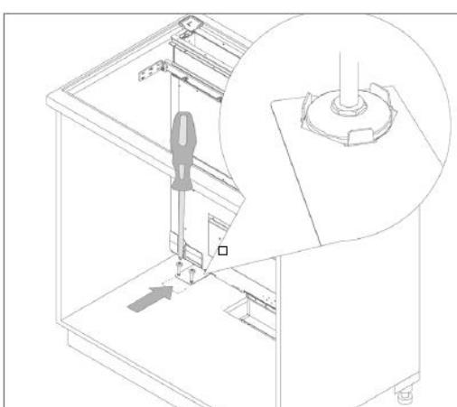
ENG Fix the levelling feet inside the cabinet.
