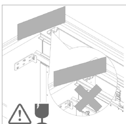
ENG Set the height of the cooker hood with a ruler, it must be levelled with the worktop (surface) or levelled with the milling edge (flush line) to prevent glass damage hob.
